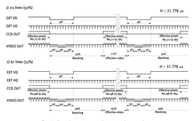
Fig. 11. Partial scanning vertical timing with external sync
